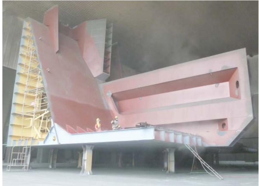
**Ship block under blasting process**
