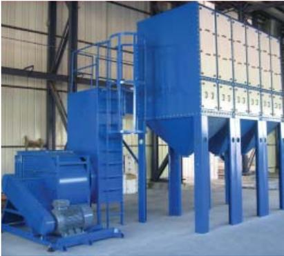
**High efficiency Blasttechnik TDF ventilation dust collector ensures correct amount of air changes per hour are achieved within the blasting chamber**
